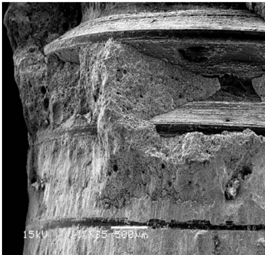
Fig. 9 SEM micrograph of fracture surface of polymeric threaded FRC device after push-out test. Fracture occurred through outer layer of FRC threads, suggesting that main reason for failure was low cohesive shear strength of plaster. (Original magnification \times 35 )
